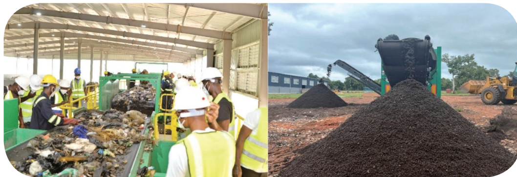
Figure 4.8 Manual sorting of municipal solid waste and compost materials on the conveyor belt
